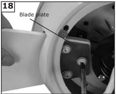
Align the blade and then the blade plate with castings on motor to attach blades to motor.
